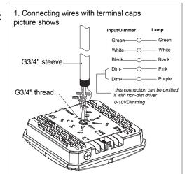
2. Rotating the steeve to make it fixed with lam Installation completed.
