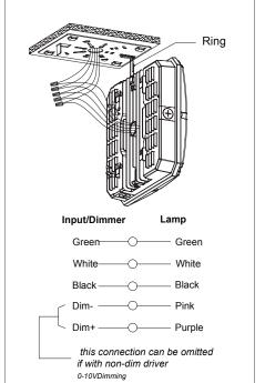
Installation method II: Pole-pendent Installation
