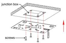
5. Secure the screw. Installation complete
