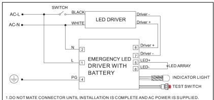
1.DO NOT MATE CONNECTOR UNTIL INSTALLATION IS COMPLETE AND AC POWER IS SUPPLIED. 2.TEST ACCESSORY LEADS-OBSERVE PROPER POLARITY WIRING.
